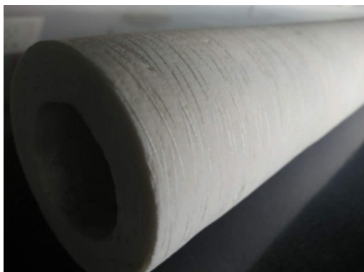
图 7 连续纤维缠绕陶瓷纤维过滤材料 Figure 7 Continuous fiber winding ceramic fiber filter materials
